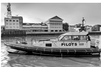
The Port of London Authority's new electric/hybrid ORC 136e pilot boat. It is the first of its kind in the UK, and is capable of sailing with 300kW of electric propulsion.
